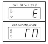
"M" for "Metric" (kilometers). Press the SPEED "+" button to change the unit of measurement. Remove and then reinsert the key.
